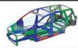
High Tensile Strength Steel 980 MPa class 590 MPa class 440 MPa class
